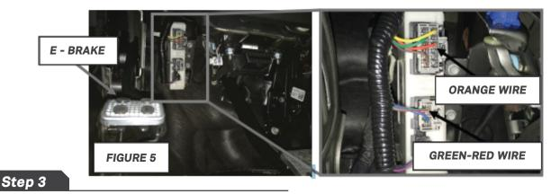
Attach 6" wire between ORANGE wire (pin 3 on C2498C connector and GREEN-RED wire (on F150) or RED wire (on Super Duty) (Pin 1 on C2498A connector) using Scotch-locks (for F150 supplied scotch-locks can be used, Super Duty are not supplied, recommend using 3M 902). This will activate a continuous +12V to the +12V power pin on the 7 pin trailer connector. Refer to figure 6.
