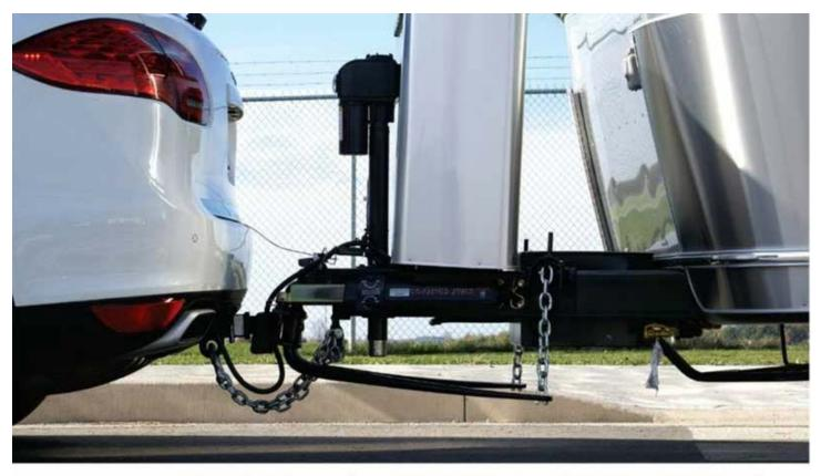
When properly adjusted, the torsion bars and sway control will produce a smooth, stable, and level rig.
