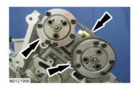
76. *NOTICE:* The front camshaft bearing mega cap must be removed first and then the remaining camshaft bearing caps. Failure to follow this direction may result in damage to the engine.
