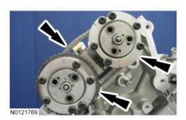
51. *NOTICE:* The front camshaft bearing mega cap must be removed first and then the remaining camshaft bearing caps. Failure to follow this direction may result in damage to the engine.
