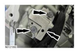
69. **NOTE:** It may be necessary to rotate the crankshaft slightly to provide enough slack in the chain to remove the LH timing chain tensioner arm. Return the crankshaft keyway to the 9 o'clock position after removing the LH timing chain tensioner arm.
