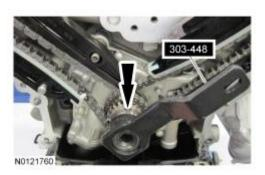
33. Verify the data matrix on the camshafts is facing up, if not, rotate the crankshaft clockwise one revolution.
