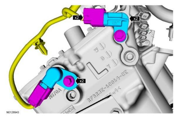
62. Detach the wiring harness retainer from the LH cylinder head.
