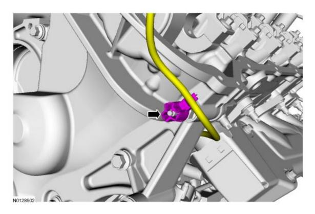
20. Remove the nut and the ground wire from the engine front cover stud bolt.
