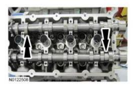
55. Remove the 16 camshaft roller follower and hydraulic lash adjuster assemblies.
