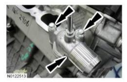
60. Remove the 2 bolts and the heat shield from the LH cylinder head.
