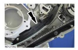
70. **NOTE:** It may be necessary to rotate the crankshaft slightly to provide enough slack in the chain to remove the LH timing chain guide. Return the crankshaft keyway to the 9 o'clock position after removing the LH timing chain guide.
