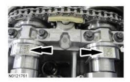
34. Remove the 2 bolts and the RH primary timing chain tensioner.
