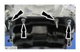
28. Remove the engine front cover-to-oil filter adapter bolt.
