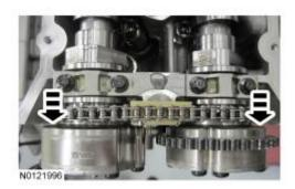
74. Depress the LH secondary timing chain tensioner and turn the tensioner 90 degrees.
