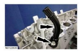
39. Remove the bolt, stud bolt and heat shield from the RH cylinder head.
