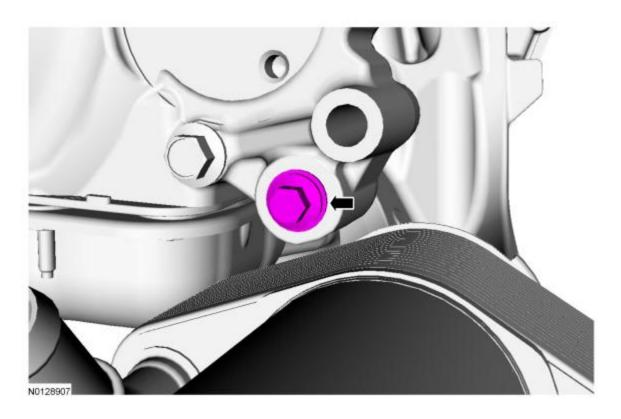
29. Using a 10 mm (0.393 in) Hex Bit loosen the engine front cover-to-oil filter adapter jack screw.
