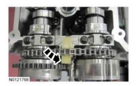
50. Remove the RH <u>VCT</u> assemblies and the RH secondary timing chain.
