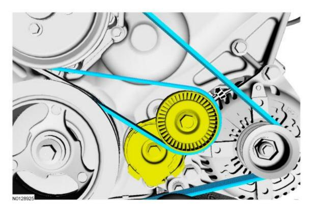
15. Rotate the A/C compressor belt tensioner clockwise and remove the A/C compressor belt.
