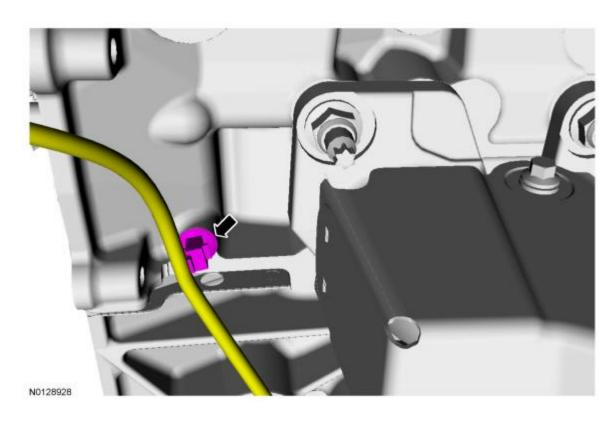
63. Remove the 3 bolts and the LH exhaust manifold heat shield.
