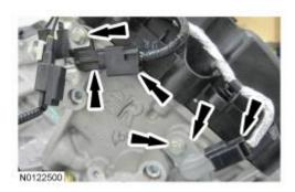
41. Disconnect the Cylinder Head Temperature (CHT) sensor electrical connector.
