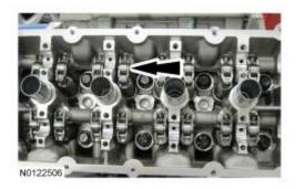
56. *NOTICE:* The cylinder head must be cool before removing it from the engine. Cylinder head warpage can result if a warm or hot cylinder head is removed.
