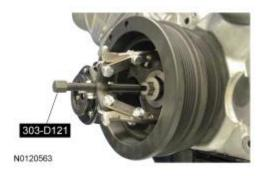
25. *NOTICE:* Use care not to damage the engine front cover or the crankshaft when removing the seal.
