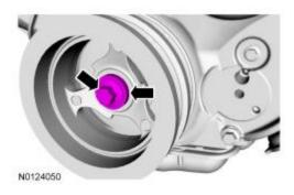
24. Using the 3 Jaw Puller and the crankshaft pulley bolt, remove the crankshaft pulley.Discard the crankshaft pulley bolt.
