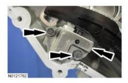
35. **NOTE:** It may be necessary to rotate the crankshaft slightly to provide enough slack in the chain to remove the RH timing chain tensioner arm. Return the crankshaft keyway to the 12 o'clock position after removing the RH timing chain tensioner arm.
