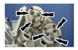
73. Slide the LH <u>VCT</u> assemblies and secondary timing chain forward 2 mm (0.078 in).
