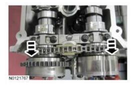
49. Depress the RH secondary timing chain tensioner and turn the tensioner 90 degrees.
