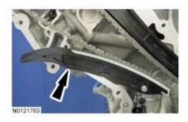
36. **NOTE**: It may be necessary to rotate the crankshaft slightly to provide enough slack in the chain to remove the RH timing chain guide. Return the crankshaft keyway to the 12 o'clock position after removing the RH timing chain guide.
