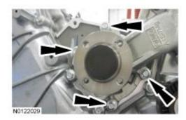
18. Remove the bolt and the accessory drive belt tensioner.
