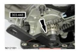
68. Remove the 2 bolts and the LH primary timing chain tensioner.
