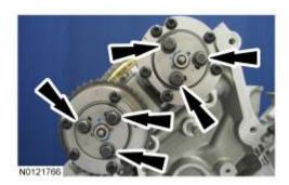
48. Slide the RH VCT assemblies and secondary timing chain forward 2 mm (0.078 in).
