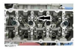
81. *NOTICE:* The cylinder head must be cool before removing it from the engine. Cylinder head warpage can result if a warm or hot cylinder head is removed.
