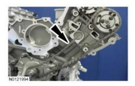
72. Remove the 3 LH intake Variable Camshaft Timing (VCT) assembly bolts and the 3 LH exhaust  $\underline{\text{VCT}}$  assembly bolts.
