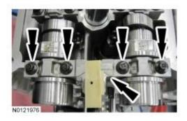
52. Remove the 16 bolts and the 8 camshaft bearing caps.
