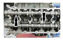
80. Remove the 16 camshaft roller follower and hydraulic lash adjuster assemblies.
