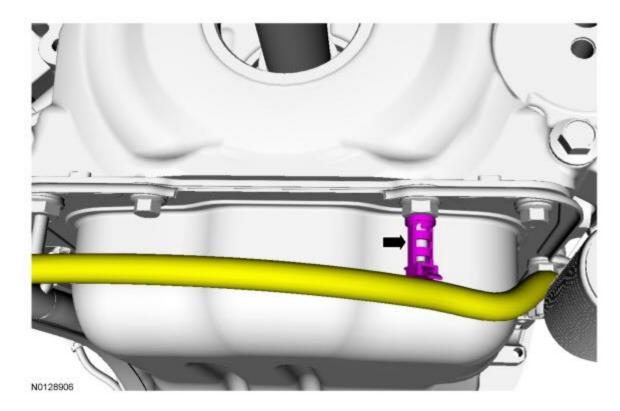
27. Remove the 2 front oil pan stud bolts and 2 front oil pan bolts.
