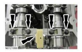
77. Remove the 16 bolts and the 8 camshaft bearing caps.
