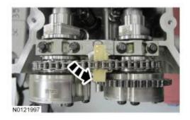
75. Remove the LH <u>VCT</u> assemblies and the LH secondary timing chain.
