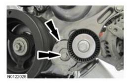
19. Detach the wiring harness retainer from the engine front cover stud bolt.
