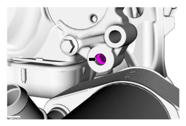
30. Remove the 13 engine front cover bolts and the 2 stud bolts.
