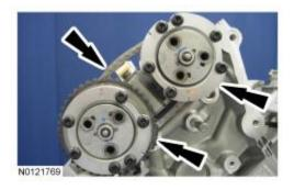
12. Using the crankshaft holding tool, rotate the crankshaft counterclockwise until the crankshaft keyway is at the 9 o'clock position.
