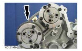
17. **NOTE:** It may be necessary to rotate the exhaust camshaft slightly (using a wrench on the flats of the camshaft) to seat the <u>VCT</u> assemblies onto the camshafts.
