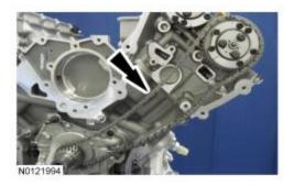
17. Remove the 3 LH intake Variable Camshaft Timing (VCT) assembly bolts and the 3 LH exhaust <u>VCT</u> assembly bolts.
