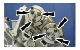
18. Slide the LH <u>VCT</u> assemblies and secondary timing chain forward 2 mm (0.078 in).
