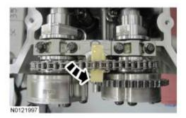
20. Remove the LH VCT assemblies and the LH secondary timing chain.
