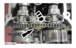
18. **NOTE:** Use a wrench on the flats of the camshaft to hold the camshafts while tightening the <u>VCT</u> assembly bolts.
