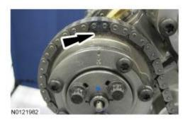
20. Align the remaining colored link on the timing chain with the timing mark on the crankshaft sprocket.
