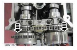
10. Depress the RH secondary timing chain tensioner and turn the tensioner 90 degrees.
