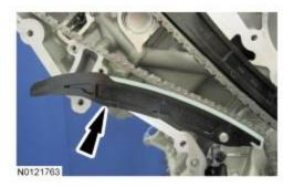
6. **NOTE:** It may be necessary to rotate the crankshaft slightly to provide enough slack in the chain to remove the RH timing chain guide. Return the crankshaft keyway to the 12 o'clock position after removing the RH timing chain guide.
