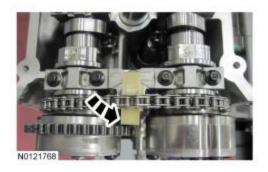
11. Remove the RH <u>VCT</u> assemblies and the RH secondary timing chain.
