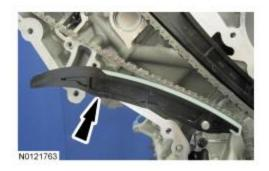
23. *NOTICE:* IF EITHER THE PRIMARY TENSIONER OR TIMING CHAIN TENSIONER ARM REQUIRE REPLACEMENT, BOTH THE PRIMARY TENSIONER AND TIMING CHAIN TENSIONER ARM MUST BE REPLACED. FAILURE TO REPLACE BOTH THE PRIMARY TENSIONER AND TIMING CHAIN TENSIONER ARM MAY RESULT IN OVERLOADING OF THE TIMING CHAIN AND UNDER CERTAIN CONDITIONS COULD LEAD TO TIMING CHAIN FAILURE.
