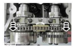
19. Depress the LH secondary timing chain tensioner and turn the tensioner 90 degrees.
