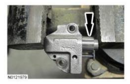
11. Using a small screwdriver or pick, push back and hold the ratchet mechanism, then push the ratchet arm back into the tensioner housing.
