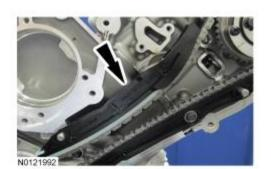
Remove the LH timing chain tensioner arm.
