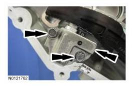
5. **NOTE:** It may be necessary to rotate the crankshaft slightly to provide enough slack in the chain to remove the RH timing chain tensioner arm. Return the crankshaft keyway to the 12 o'clock position after removing the RH timing chain tensioner arm.
