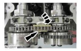
5. **NOTE:** Use a wrench on the flats of the camshaft to hold the camshafts while tightening the <u>VCT</u> assembly bolts.
