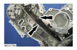
22. NOTICE: IF EITHER THE PRIMARY TENSIONER OR TIMING CHAIN TENSIONER ARM REQUIRE REPLACEMENT, BOTH THE PRIMARY TENSIONER AND TIMING CHAIN TENSIONER ARM MUST BE REPLACED. FAILURE TO REPLACE BOTH THE PRIMARY TENSIONER AND TIMING CHAIN TENSIONER ARM MAY RESULT IN OVERLOADING OF THE TIMING CHAIN AND UNDER CERTAIN CONDITIONS COULD LEAD TO TIMING CHAIN FAILURE.
