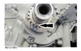
21. **NOTE:** It may be necessary to rotate the crankshaft slightly to provide enough slack in the chain to install the RH timing chain guide. Return the crankshaft keyway to the 12 o'clock position after installing the RH timing chain guide.
