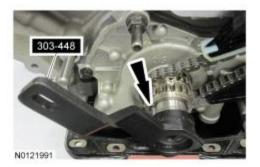
13. *NOTICE:* IF EITHER THE PRIMARY TENSIONER OR TIMING CHAIN TENSIONER ARM REQUIRE REPLACEMENT, BOTH THE PRIMARY TENSIONER AND TIMING CHAIN TENSIONER ARM MUST BE REPLACED. FAILURE TO REPLACE BOTH THE PRIMARY TENSIONER AND TIMING CHAIN TENSIONER ARM MAY RESULT IN OVERLOADING OF THE TIMING CHAIN AND UNDER CERTAIN CONDITIONS COULD LEAD TO TIMING CHAIN FAILURE.
