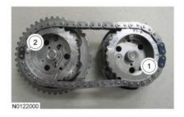
Install the LH <u>VCT</u> assemblies and the secondary timing chain onto the LH camshafts to a position 2 mm (0.078 in) from fully seated. The timing mark on the exhaust <u>VCT</u> assembly should be in the 11 o'clock position.
