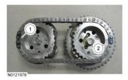
Install the RH <u>VCT</u> assemblies and the secondary timing chain onto the RH camshafts to a position 2 mm (0.078 in) from fully seated. The timing mark on the exhaust <u>VCT</u> assembly should be in the 1 o'clock position.
