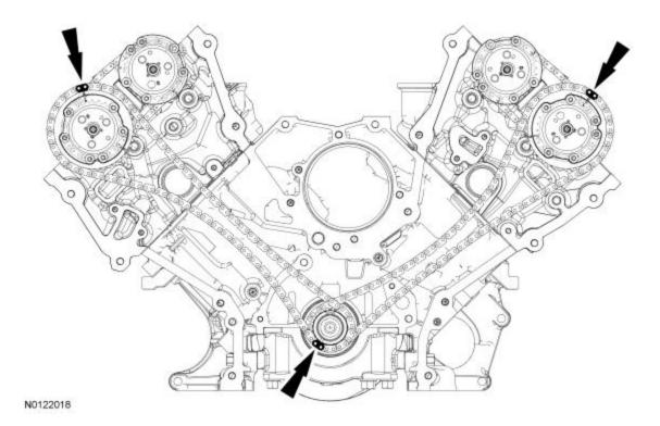
25. Install the engine front cover. For additional information, refer to Engine Front Cover in this section.
