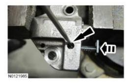
12. Install a suitable pin into the hole of the tensioner housing to hold the ratchet assembly and plunger in place during installation.
