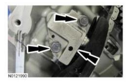
14. *NOTICE:* IF EITHER THE PRIMARY TENSIONER OR TIMING CHAIN TENSIONER ARM REQUIRE REPLACEMENT, BOTH THE PRIMARY TENSIONER AND TIMING CHAIN TENSIONER ARM MUST BE REPLACED. FAILURE TO REPLACE BOTH THE PRIMARY TENSIONER AND TIMING CHAIN TENSIONER ARM MAY RESULT IN OVERLOADING OF THE TIMING CHAIN AND UNDER CERTAIN CONDITIONS COULD LEAD TO TIMING CHAIN FAILURE.
