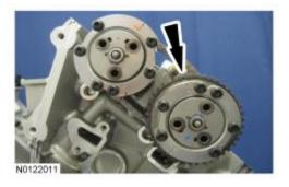
4. **NOTE:** It may be necessary to rotate the exhaust camshaft slightly (using a wrench on the flats of the camshaft) to seat the <u>VCT</u> assemblies onto the camshafts.
