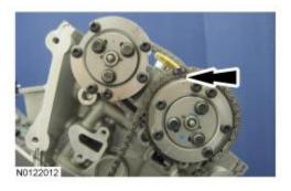
7. Align the remaining colored link on the timing chain with the timing mark on the crankshaft sprocket.
