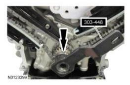
3. Verify the data matrix on the camshafts is facing up, if not, rotate the crankshaft clockwise one revolution.
