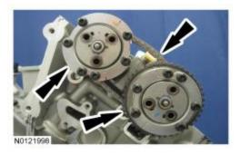
21. Remove the crankshaft sprocket.
