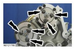
9. Slide the RH <u>VCT</u> assemblies and secondary timing chain forward 2 mm (0.078 in).
