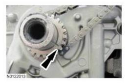
8. **NOTE:** It may be necessary to rotate the crankshaft slightly to provide enough slack in the chain to install the LH timing chain guide. Return the crankshaft keyway to the 9 o'clock position after installing the LH timing chain guide.
