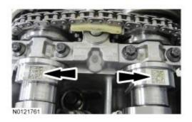
4. Remove the 2 bolts and the RH primary timing chain tensioner.
