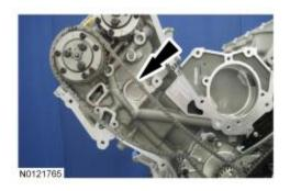
8. Remove the 3 RH intake Variable Camshaft Timing (VCT) assembly bolts and the 3 RH exhaust <u>VCT</u> assembly bolts.
