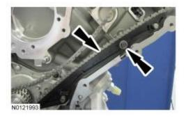
9. *NOTICE:* IF EITHER THE PRIMARY TENSIONER OR TIMING CHAIN TENSIONER ARM REQUIRE REPLACEMENT, BOTH THE PRIMARY TENSIONER AND TIMING CHAIN TENSIONER ARM MUST BE REPLACED. FAILURE TO REPLACE BOTH THE PRIMARY TENSIONER AND TIMING CHAIN TENSIONER ARM MAY RESULT IN OVERLOADING OF THE TIMING CHAIN AND UNDER CERTAIN CONDITIONS COULD LEAD TO TIMING CHAIN FAILURE.
