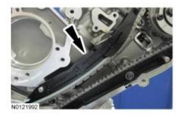
Install the LH timing chain tensioner arm.
