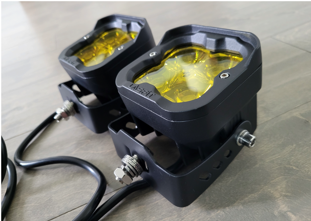
Universal mounting brackets installed
