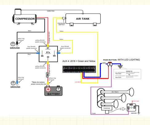
Using an upfitter AUX switch to power the pressure sensor 12v lead as well as the 12v side of the Push Button (and LED if equipped) enables deactivation of entire air and horn system with the flip of the AUX switch.
