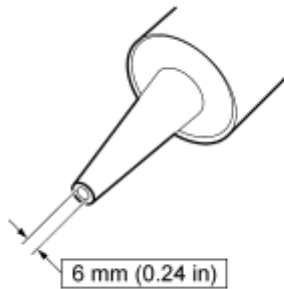
Fig. 74: Cutting Urethane Adhesive Applicator Tip To Specification Courtesy of FORD MOTOR CO.
