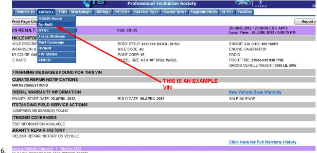
7. They cannot add or change as built data to any of the other modules. Just the DSM. All other module as built data needs to be from the original VIN.
