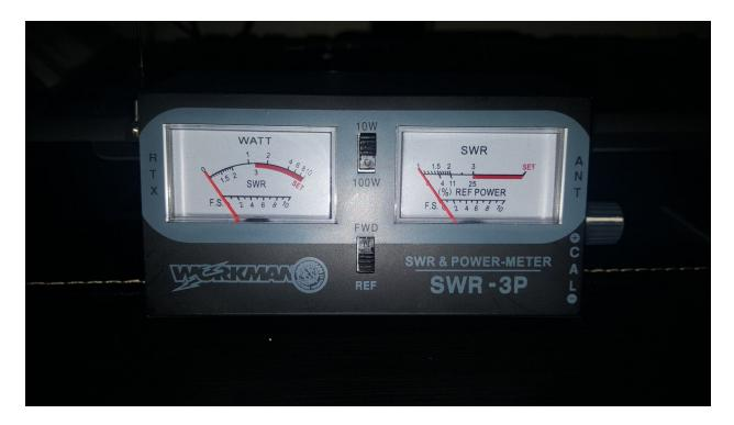
Radio, meter and antenna in hand i went to an open field to start my testing and it is here where i ran into my next big problem. Because i has used the 3m rubber barrier to avoid galvanic corrosion i had also stripped my system of a ground plane. The SWR meter would shoot up past 5 which is a solid NO-GO for CB operation. You want an SWR lower than 2 and the closer to 1:1 the better.
