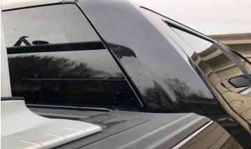
Good news, there is no need to worry, with some measuring and an exacto knife you can cut through the plastic and expose the stake hole pockets.
