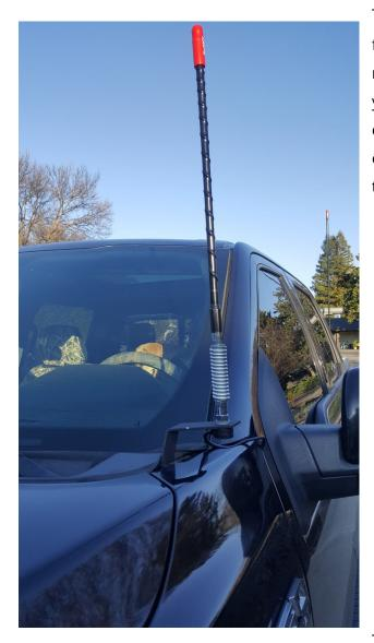
This is where the next project would sprout from. I wanted to integrate a dual band radio into my truck next. Now a couple years have passed and an awesome company called Procomm has launched an easy way to mount and ground an antenna to your 2015 or newer F-150.
