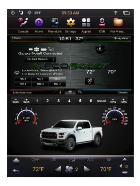
The top half of the screen displays the SYNC system (in my case SYNC2) and is fully functional and operates the same way as before the PX6 unit was installed. The bottom help is a static display that can't be changed, but the RPM and MPG meters are active.
