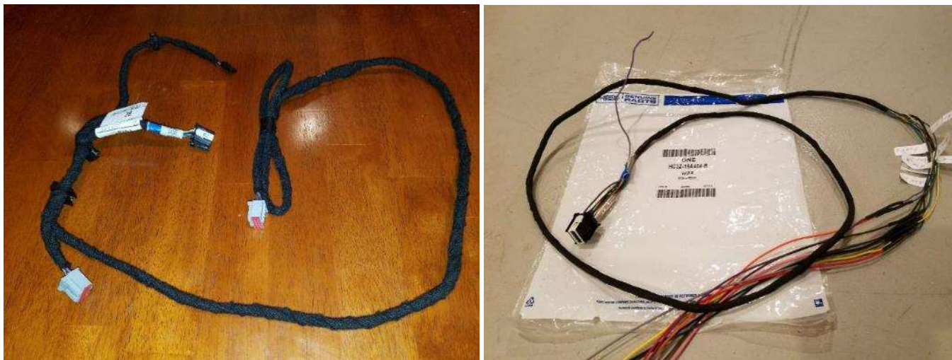
Figure 2 - Console Wiring Harness (HC3Z-15A404-B) Unpacked, and after modification with extra connectors removed and wires extended. Partially taped.
