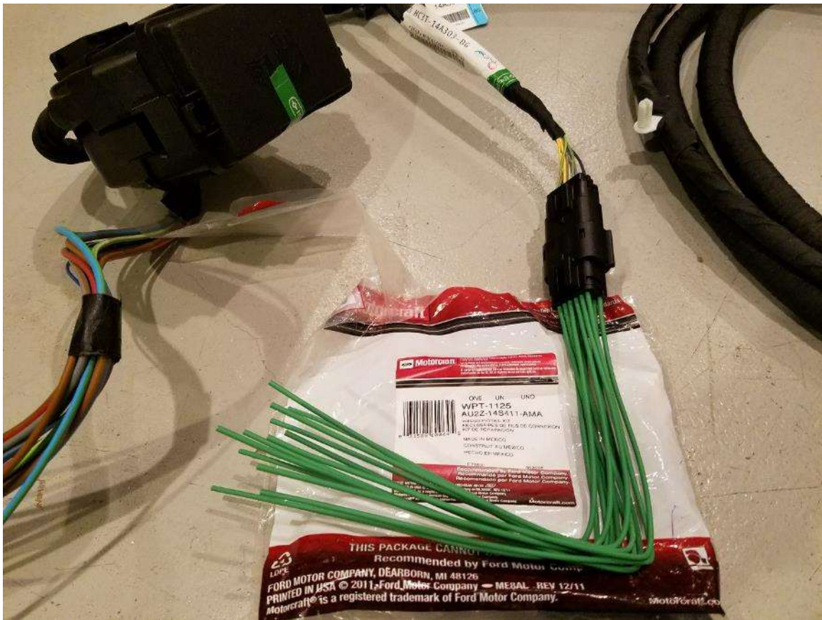
Figure 9 - Pigtail WPT-1125 Connected to Relay Box Connector
