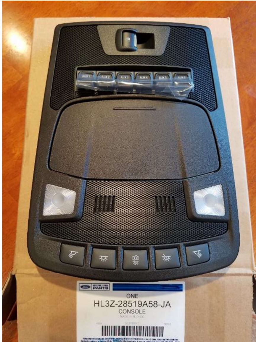
Figure 3 - CONSOLE ASY - OVERHEAD (HL3Z-28519A58-JA)
