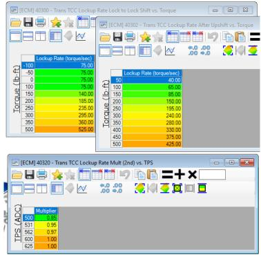
For #2, set all of the cells in the tables to 0 for each of the gears. The same goes for Min Slip Upshift / Downshift.
