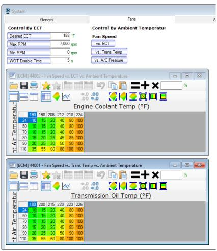
Here are some changes I made that I've been experimenting with my Reische Ford-4D 170F thermostat. Reische doesn't have any recommended settings for the newer EcoBoost and Coyote Fords because the settings are different from what were used on the older modular engines (High Fan On/Off and Low Fan On/Off).
