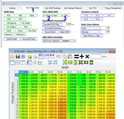
Basically rows 9 and higher is at WOT. The downshift mapping seemed confusing at first, but basically the highest values (the last 2 rows) seem to be the limit at which you can manually downshift into that gear. I don't recommend changing these values other than perhaps raising the upshift values at rows 9 and above. You can calculate OSS based on gearing, tire size, etc... I have a spreadsheet that does this, but I found that this table has little impact on WOT shift RPMs.
