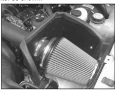
34. Install the K&N® air filter assembly onto the K&N® intake tube as shown and secure with the provided hose clamp.
