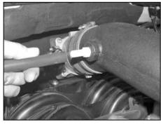
30. Install the provided silicone vent hose onto the valve cover and onto the K&N<sup>®</sup> intake tube as shown.
