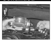
11. Lift the throttle body from the intake manifold and disconnect throttle body motor electrical connection.
