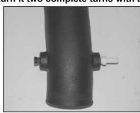
24a. On vehicles that are equipped with only one vent line, install the provided NPT plug as shown.
