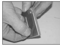
20. Install the provided gasket onto the K&N® mass air adapter as shown; sticky side down.
