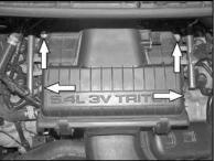
Remove the four air box mounting bolts shown with a 10mm socket.
