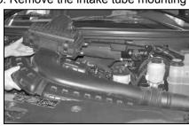
6. Remove the entire intake tube & air filter assembly from the vehicle.
