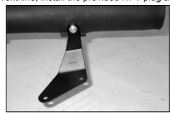
25. Install the tube mounting bracket (070118) onto the  $K\&N^{\circledcirc}$  intake tube as shown with the provided hardware.
