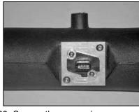
23. Secure the mass air sensor assembly onto the  $K\&N^{\circledcirc}$  intake tube with the provided hardware as shown.
