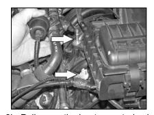
3b. Pull up on the heater control valve and wiring harness mounting clips to unhook them from the air box mounting studs as shown.
