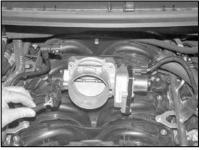
14. Reconnect the throttle body motor and the TPS electrical connection.
