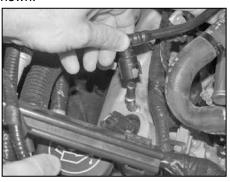
29. Unlock the crank case vent hose and remove the hose from the valve cover.
