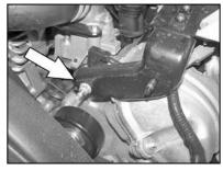
8. On vehicles that are equipped with the intake tube support bracket, reinstall one of the 13mm nuts removed in step #7 onto the lower mounting stud and tighten.
