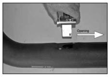
22. Install the mass air sensor assembly into the K&N® intake tube.
