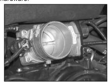
26. Install silicone hose (#08630) onto the throttle body with the provided hose clamps as shown.
