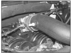
27. Install the K&N $^{\circ}$  intake tube into the silicone hose and then tighten the provided hose clamp.
