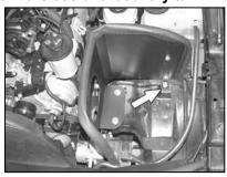
18. Install the heatshield as shown and secure with the provided hardware.
