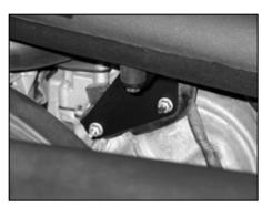
28. Connect the K&N® intake tube to the bracket with the provided hardware as shown.
