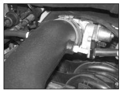
30a. On vehicles equipped, attach the factory brake booster vent hose to the K&N® intake tube as shown.
