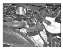
7. On vehicles that are equipped with the intake tube support bracket, remove the two 13mm nuts securing the intake tube support bracket, remove the intake tube support bracket.
