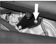
28a. On vehicles not equipped with the factory intake tube support bracket, it is necessary to use the supplied 8mm bolt, washers and nut to secure the tube mounting bracket to the engine bracket as shown.
