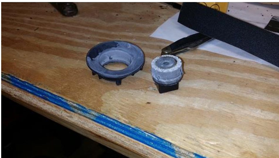
After 48 hours I cut a hole in it using a hole saw and drill press.
