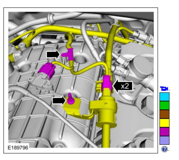
5. Install the engine appearance cover bracket and bolts. *Torque*: 89 lb.in (10 Nm)
