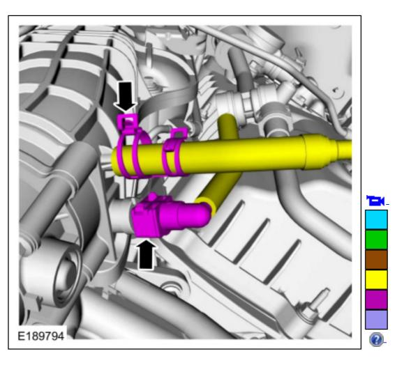
Rotate and connect the PCV tube to the intake manifold. Refer to: <u>Quick Release Coupling</u> (310-00C Fuel System - General Information - 3.5L EcoBoost (272kW/370PS), General Procedures).
