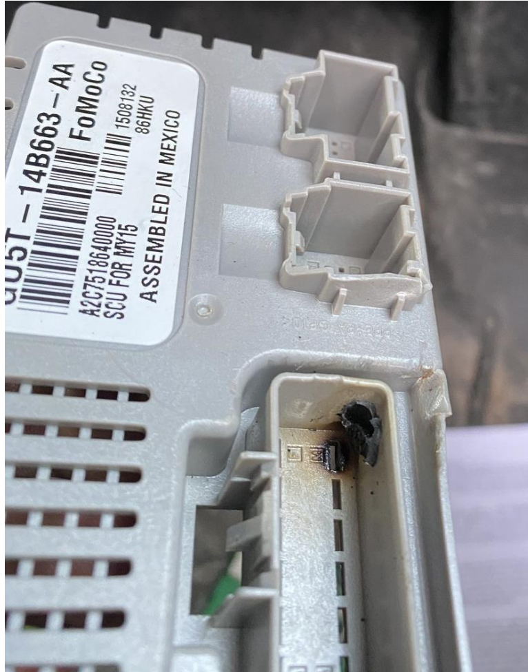
Figure 8 - SCME Damage from Terminal Failure
