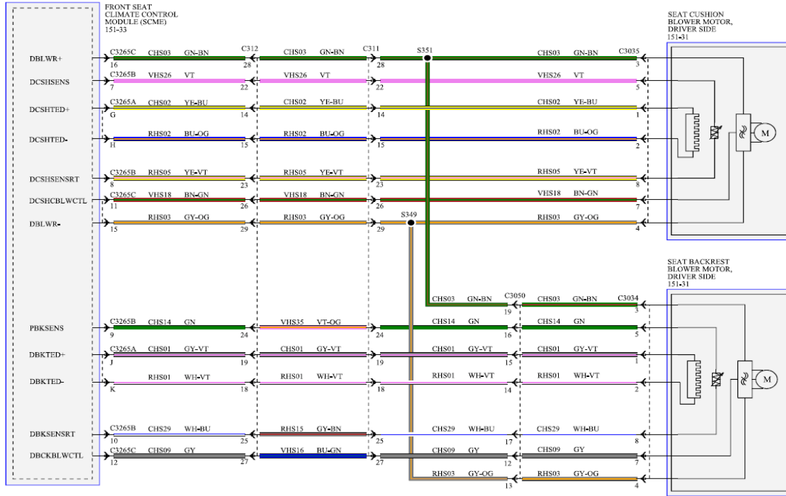
Figure 2 - Driver Side Climate Controlled Seat Wiring Diagram
