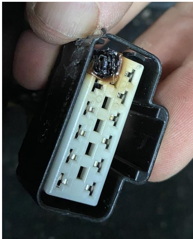
Figure 7 - Terminal Side of Connector with Failure
