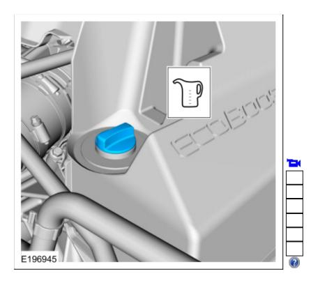
5. After filling the engine with oil, the oil must flow from the main chamber of the oil pan, through a check valve into the smaller side chamber to correctly register the oil level on the oil level indicator. This may take up to 15 minutes.
