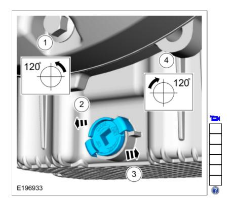
Turn the oil drain plug by hand clockwise 120 degrees.
