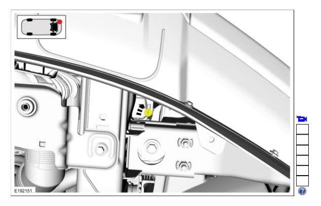
Install the vacuum cooling system filler and follow the manufacturer's instructions to fill and bleed the system.
