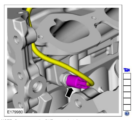
3. **NOTE**: Do not reuse the <u>CHT</u> sensor, install a new sensor.
