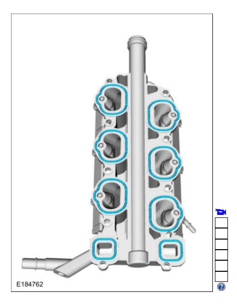
2. Install the lower intake manifold and the bolts. *Torque*: 89 lb.in (10 Nm)
