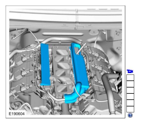
Connect the fuel tube quick release coupling. Refer to: <u>Quick Release Coupling</u> (310-00B Fuel System - General Information - 3.5L Duratec (209kW/284PS), Removal and Installation).
