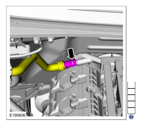
4. Connect the fuel injector electrical connectors.
