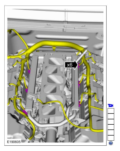
10. Disconnect the coolant tube from the lower intake manifold.
