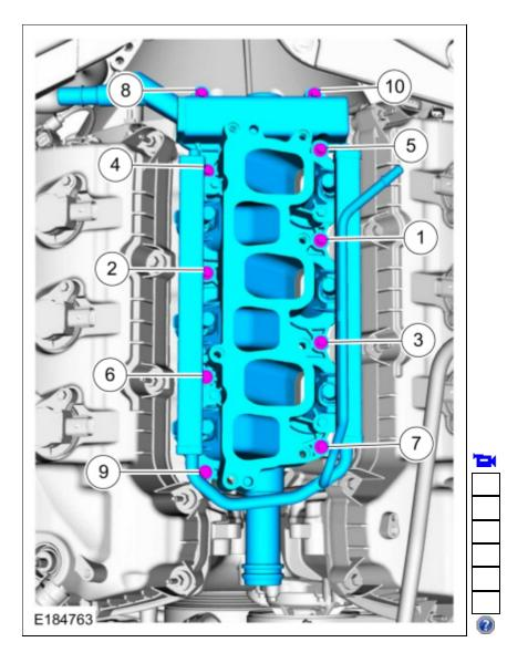
3. Connect the coolant tube to the lower intake manifold.
