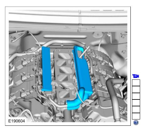
Remove the thermostat housing. Refer to: <u>Thermostat Housing</u> (303-03B Engine Cooling - 3.5L Duratec (209kW/284PS), Removal and
