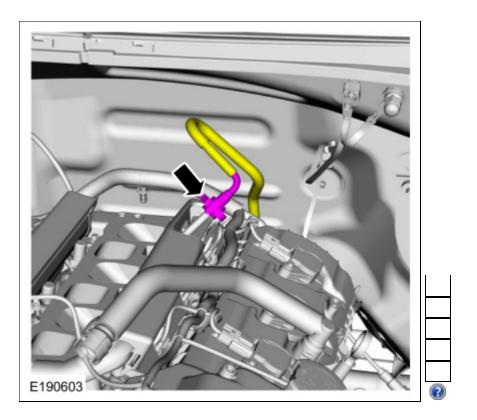
7. Remove the fuel rail sound insulators.
