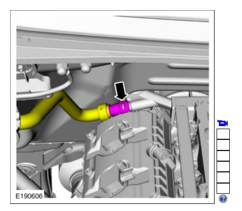
11. Remove the bolts and the lower intake manifold.
