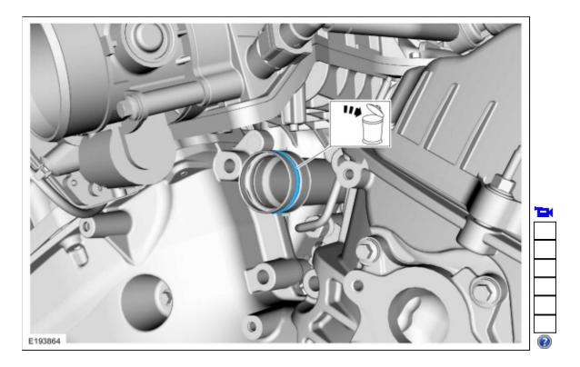
8. Inspect the O-ring seal and replace if necessary.
