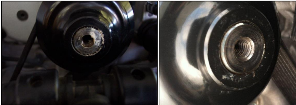
Figure 27: OEM Drive Pulley | Left: Untampered | Right: Tampered With
