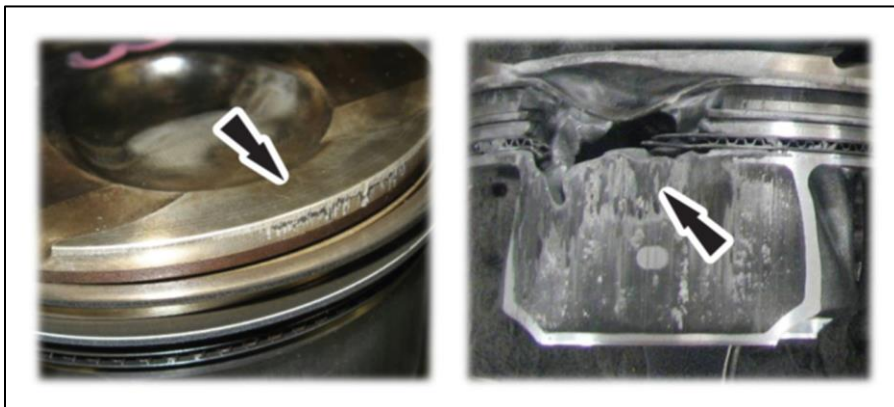
Figure 3: Light/Heavy Knock Damage
