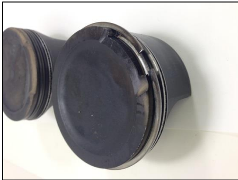
Figure 6: Ring Land Damage
