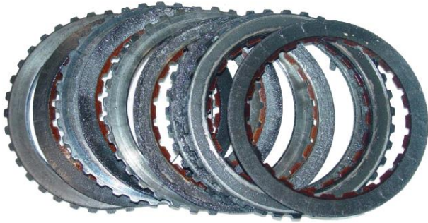
Figure 9: Damaged Clutch Discs
