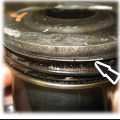
Figure 5: Piston Ring Damage
