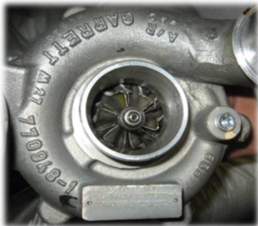
Figure 14: Compressor Blade Damage from Overspeed Event
