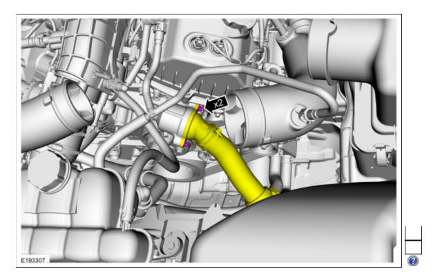
5. Remove the thermostat and discard the O-ring seal.
