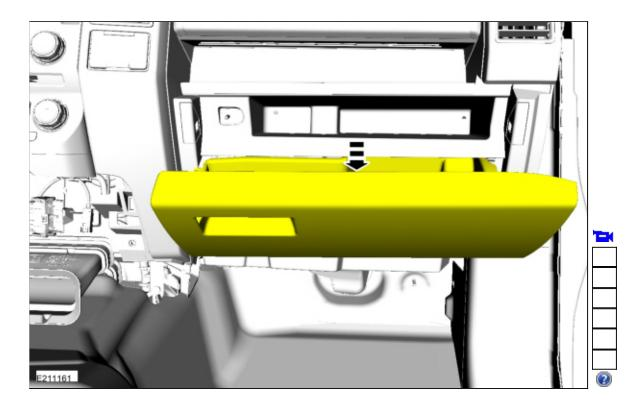
3. Remove the glove compartment dampener from the glove compartment by pushing down and forward at the damper end.
