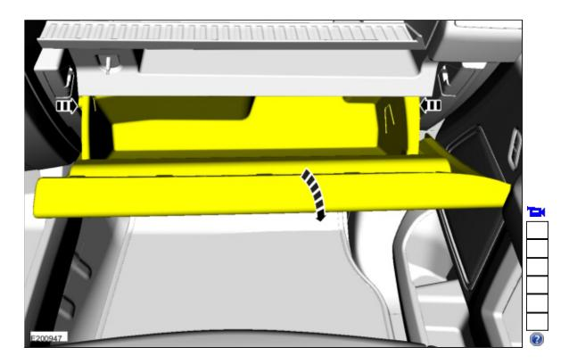
5. Remove the glove compartment from the hinge line.
