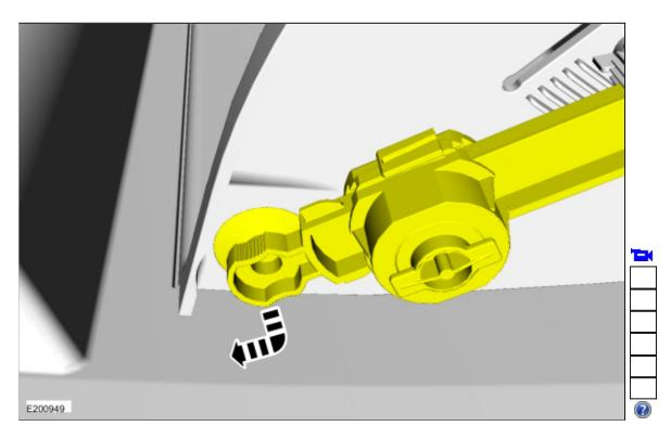
4. Release glove compartment downstops and fully lower the glove compartment.
