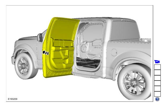
4. Loosen the bolts to permit movement of the door. Loosen:
