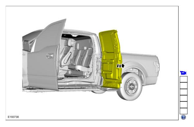
20. Tighten the bolts. *Torque*: 26 lb.ft (35 Nm)
