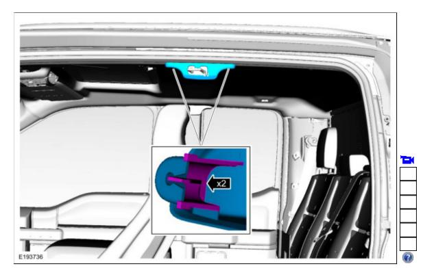
4. Remove the bolts and the upper striker assembly. *Torque*: 18 lb.ft (25 Nm)
