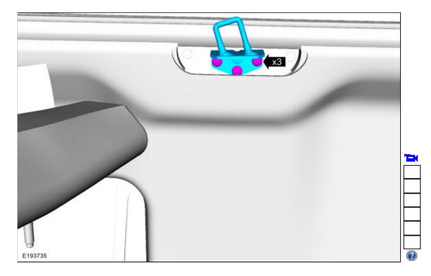
5. Remove the bolts and the lower striker assembly. *Torque*: 18 lb.ft (25 Nm)
