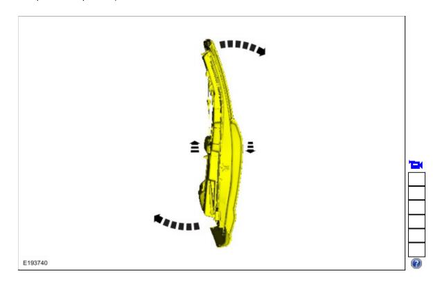
10. Tighten the bolts. *Torque*: 20 lb.ft (27.5 Nm)
