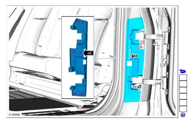
16. Loosen the bolts enough to permit movement of the door.
