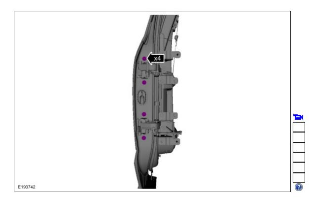
9. Adjust the door to specification. Refer to: <u>Body and Frame</u> (501-26 Body Repairs - Vehicle Specific Information and Tolerance Checks, Description and Operation).
