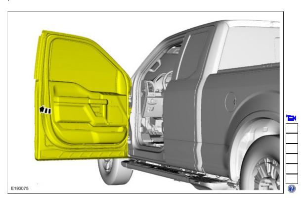
8. Loosen the bolts enough to permit movement of the door.
