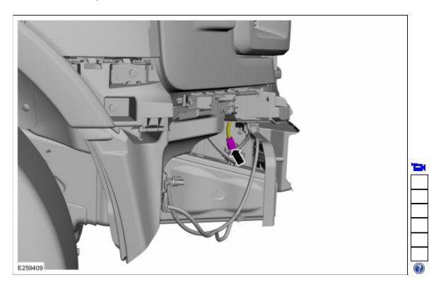
12. Remove the pin-type retainers and position aside the wire harness.
