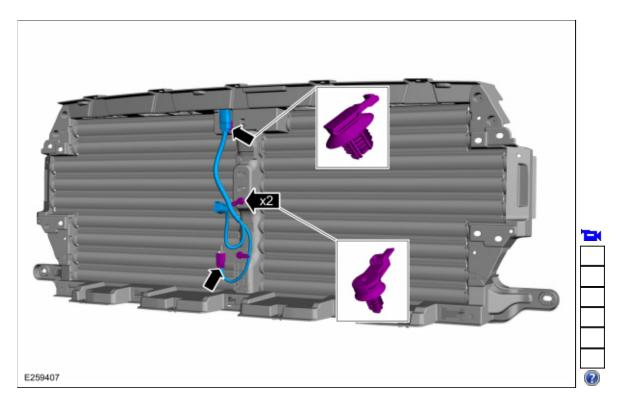
9. Remove the ambient air temperature sensor and bracket.
