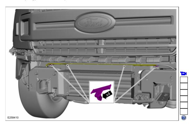
13. Remove the bolts. *Torque*: 62 lb.in (7 Nm)
