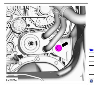
8. Install the axle shaft housing carrier bushing bolt. *Torque*: 129 lb.ft (175 Nm)
