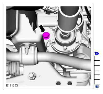
7. Install the upper front axle carrier mounting bushing bolt. *Torque*: 129 lb.ft (175 Nm)
