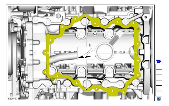
22. NOTICE: Do not use wire brushes, power abrasive discs or 3M<sup>™</sup> Roloc® Bristle Disk (2-in white, part number 07528) to clean the sealing surfaces of the engine block. These tools cause scratches and gouges that make leak paths. They also cause contamination that causes premature engine failure. Remove all traces of the gasket.
