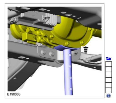
6. Install the lower front axle carrier mounting bushing bolt. *Torque*: 129 lb.ft (175 Nm)
