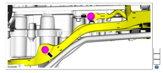
11. Remove the nut and position out the transmission cooler tube bracket. Position out the engine wiring harness.
