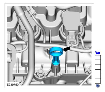
19. Fill the engine with clean engine oil.
