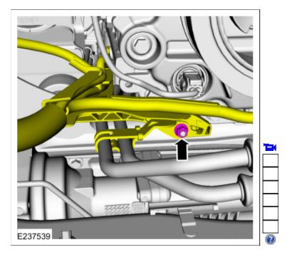
12. Attach the starter motor wiring harness retainer to the oil pan. Position the ground wire and install the bolt. *Torque*: 18 lb.ft (25 Nm)
