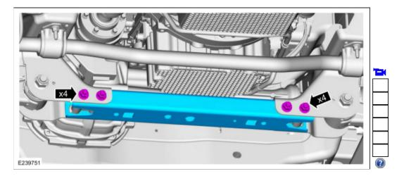
11. Position back the engine wire harness. Position back the transmission cooler tube bracket and install the nut. *Torque*: 106 lb.in (12 Nm)
