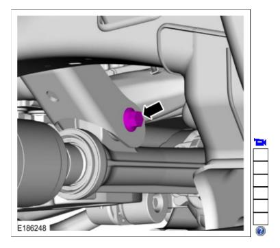
15. Remove the upper front axle carrier mounting bushing bolt.
