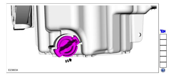
8. Remove and discard the oil filter. Use the General Equipment: Oil Drain Equipment
