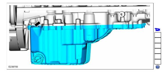
21. NOTICE: Do not use wire brushes, power abrasive discs or 3M<sup>™</sup> Roloc® Bristle Disk (2-in white, part number 07528) to clean the sealing surfaces of the engine block. These tools cause scratches and gouges that make leak paths. They also cause contamination that causes premature engine failure. Remove all traces of the gasket.
