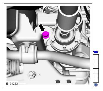
17. Using an adjustable stand, lower the axle to allow clearance for the oil pan to be removed. Use the General Equipment: Vehicle/Axle Stands
