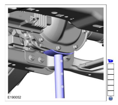
14. Remove the axle shaft housing carrier bushing bolt.
