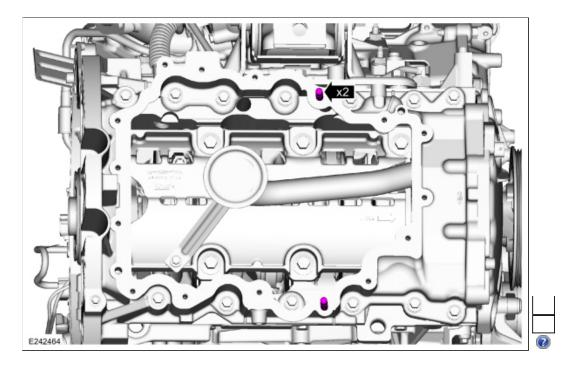
2. **NOTE:** The oil pan must be installed and the oil pan aligned to the cylinder block within 4 minutes of sealant application. Final tightening of the oil pan bolts must be carried out within 60 minutes of sealant application.
