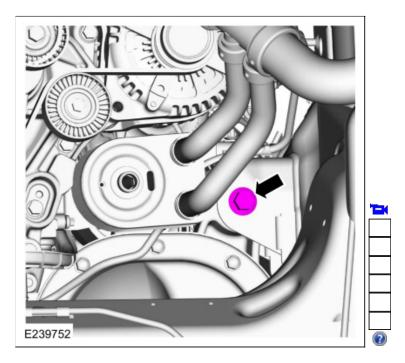
16. Remove the lower front axle carrier mounting bushing bolt.
