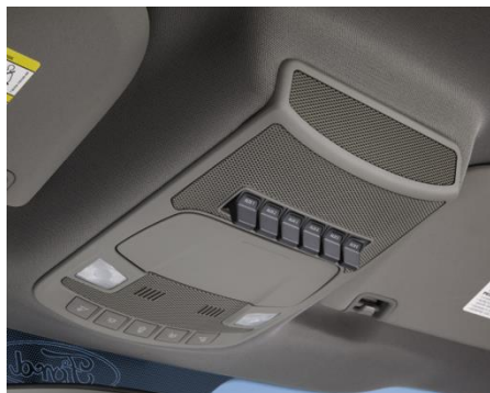
Figure 1: 2017 Super Duty Upfitter switch location
