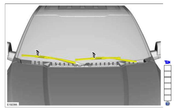
2. **NOTE:** During installation, it is necessary to fully release the windshield wiper pivot arm latch and hold while installing the pivot arm onto the wiper linkage assembly.
