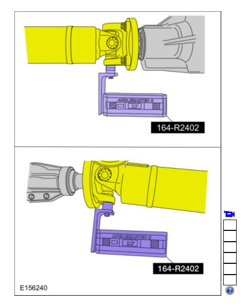
3. Special Tool(s): Anglemaster II Driveline Inclinometer/Protractor 164-R2402. Measure the slope of the connecting component. Record the measurement of the component angle as angle B.
