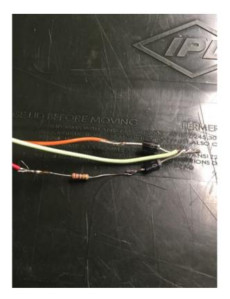
cut into the blinker wire an make connections like the diagram. Again I soldered them with shrink tube. I also used wire loom to make things neat.
