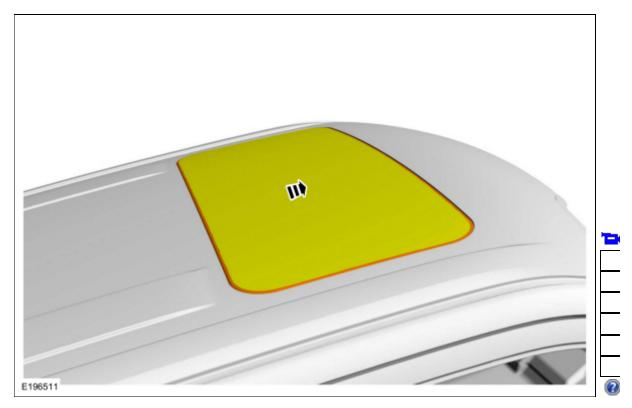
2. Measure the front and rear of the roof opening panel glass to roof clearances as shown.
