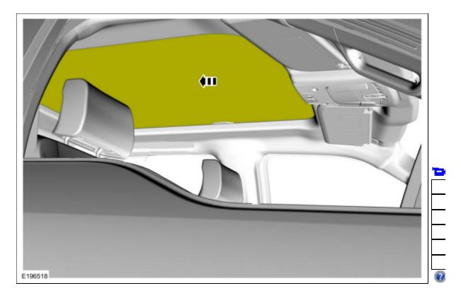
4. **NOTE:** *During installation, make sure the blind is fully seated. An audible noise will be heard when the blind seats to the lower bracket.*
