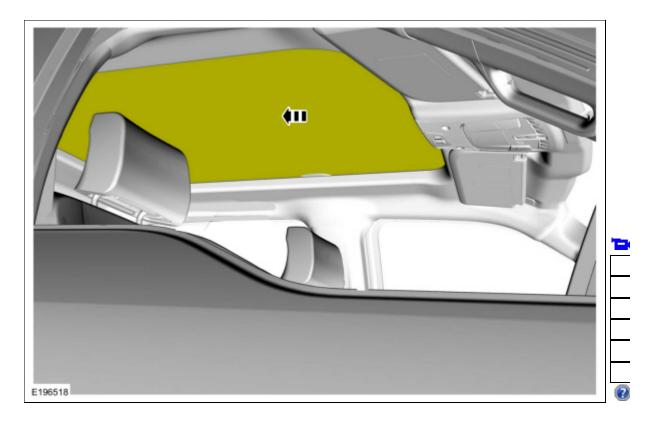
4. Adjust the roof opening panel fixed glass.
