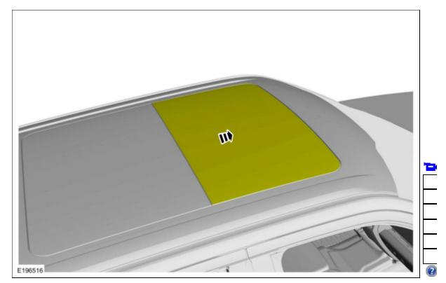
2. Measure the rear and sides of the rear fixed glass to roof clearances as shown.
