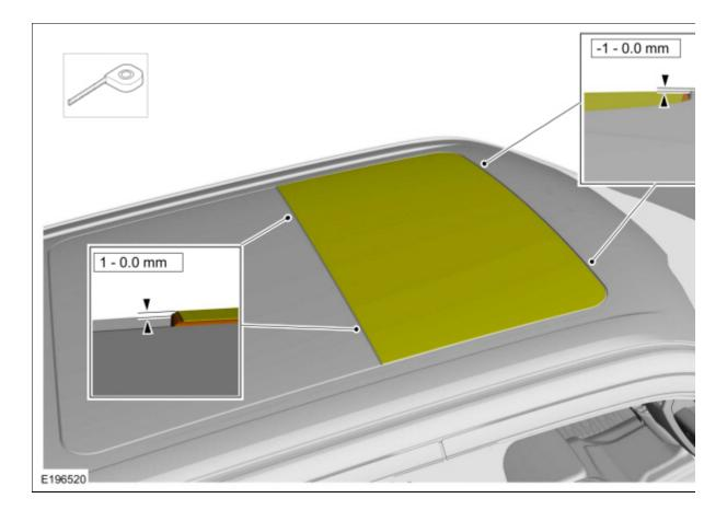
3. If adjustment is needed, fully open the roof opening panel shield.
