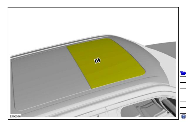
2. Measure the front of the roof opening panel sliding glass to roof clearance and the rear of the roof opening panel sliding glass to roof opening panel fixed glass as shown.
