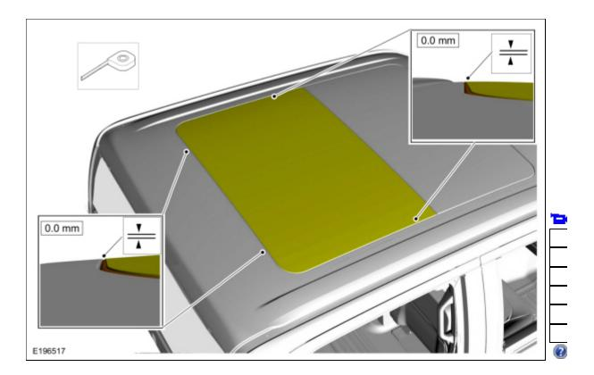
3. If adjustment is needed, fully open the roof opening panel shield.
