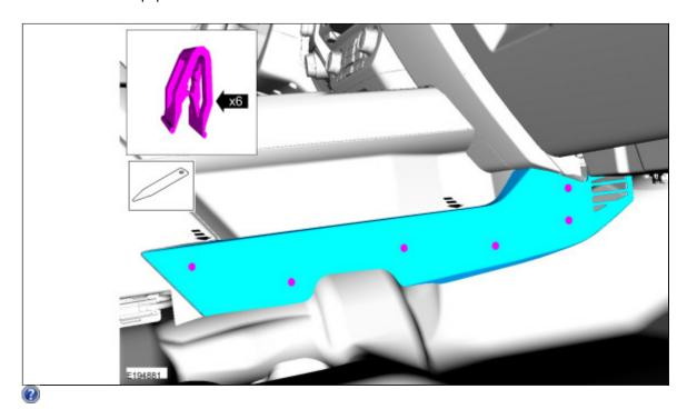
Remove the screw, release the clips and remove the <u>LH</u> lower floor console trim panel. Use the General Equipment: Interior Trim Remover *Torque*: 22 lb.in (2.5 Nm)
