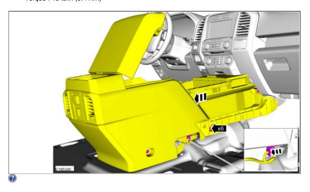
9. Disconnect the electrical connectors and remove the floor console.
