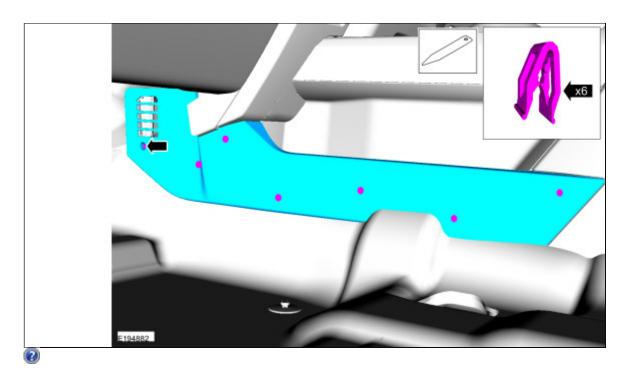
3. Remove the <u>RH finish panel</u>. Use the General Equipment: Interior Trim Remover
