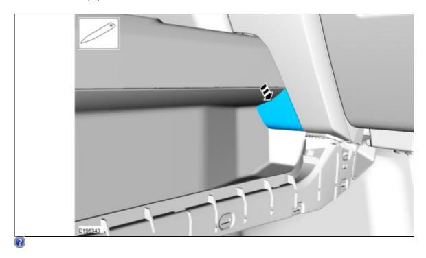
4. Remove the <u>LH finish panel</u>. Use the General Equipment: Interior Trim Remover
